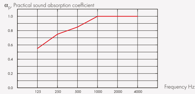
— Solo Matrix 40 mm, 300 mm o.d.s. o.d.s = overall depth of system
