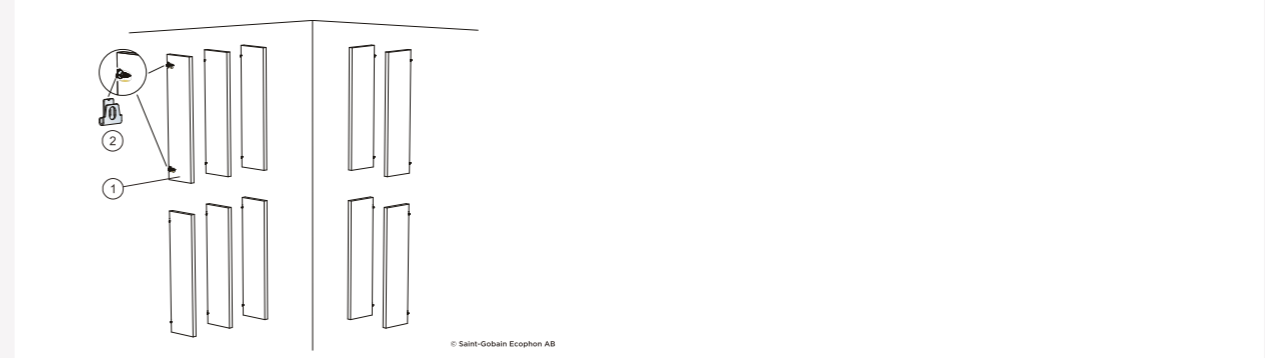
M420 Installation diagram (M420) for Ecophon Solo Baffle Wall
