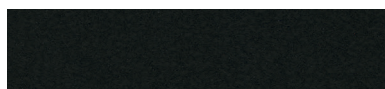
DARK DIAMOND | Light reflectance 4%. Nearest NCS colour sample S 9000-N. Grid colour NCS S 8000-N.
