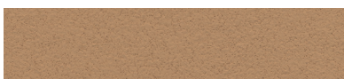
WET SAND | Light reflectance 35%. Nearest NCS colour sample S 3020-Y30R. Grid colour NCS S 3020-Y40R.
