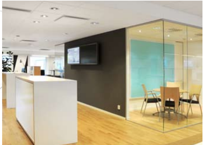
In a room with parallel, hard walls, the wall absorber removes any flutter echo.
